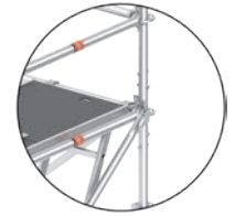
Fig. 96: Connection of vertical standards with bolted spigot
