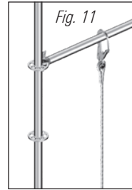
Fig. 11: Attachment to an O-ledger (U-ledger similar, where attachment is possible)
