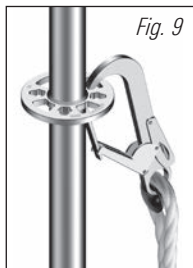
Fig. 9: Attachment in large and small hole of rosette possible (Only permissible in Allround Scaffolding in steel – not in Allround Scaffolding in aluminium)
